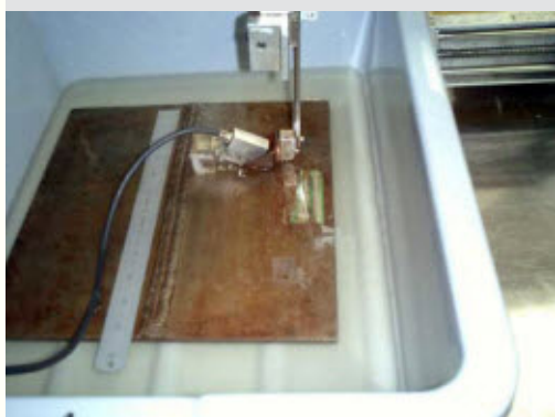
Figure 6: A phased array probe examining a half-inch weld sample in a water bath
