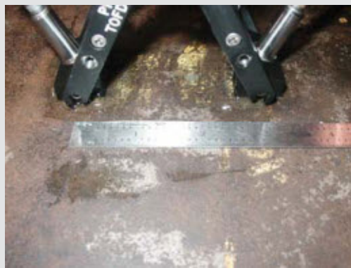
Figure 8: An example of the ToFD probes on a calibration block
